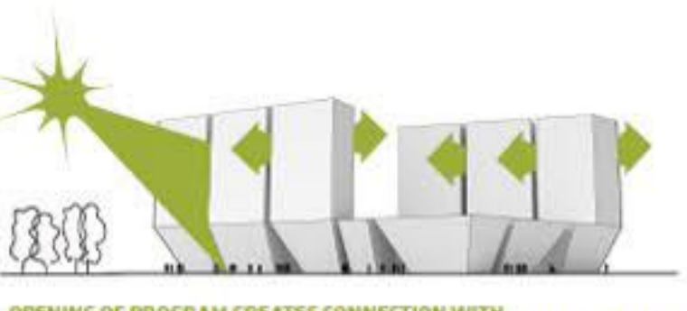
OPENING OF PROGRAM CREATES CONNECTION WITH PARK, NATURAL LIGHTING AND CROSS VENTILATION
