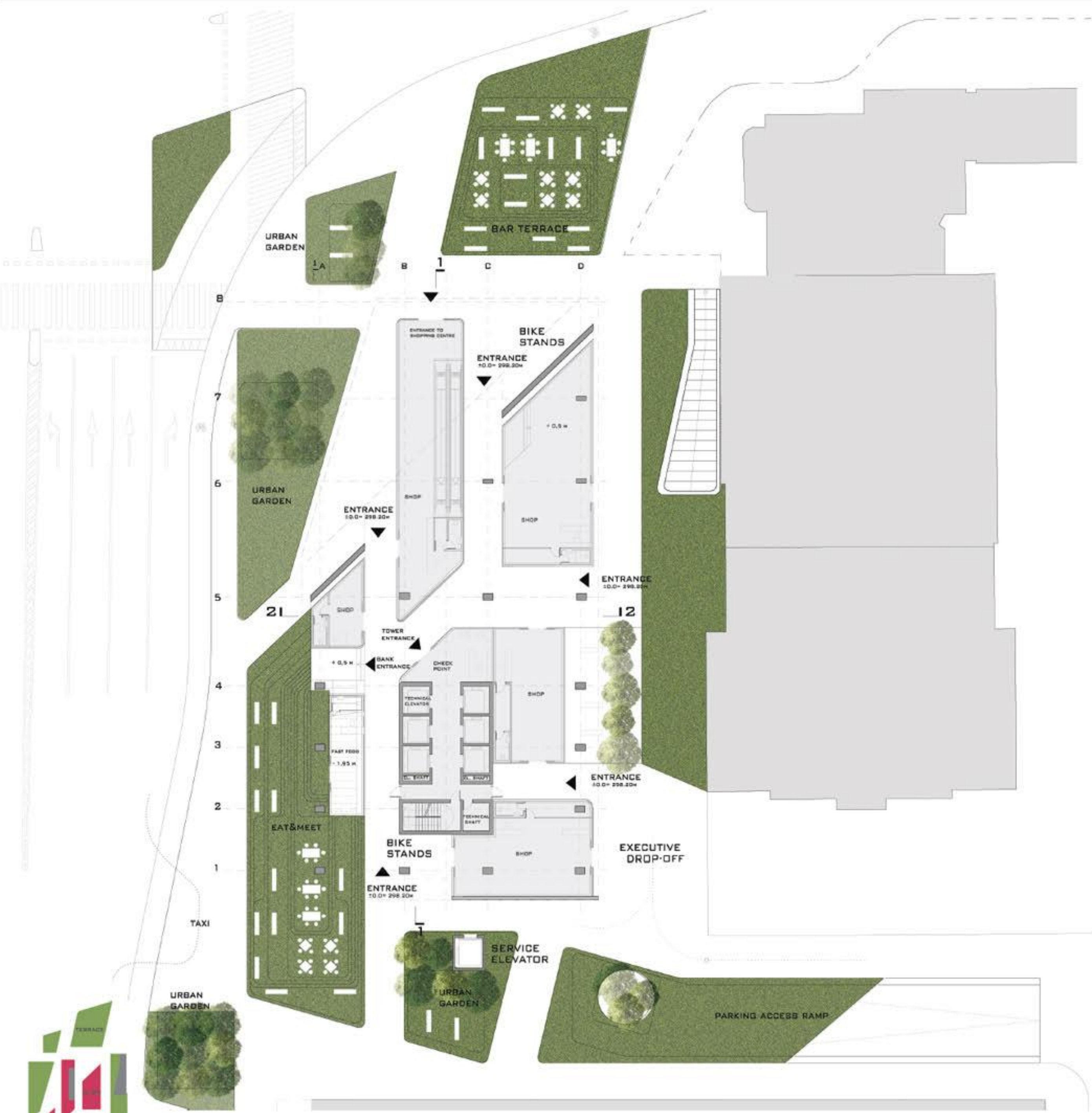
ENTRANCE STOREY / GROUND FLOOR WITH EXTERIOR ARRANGEMENT, 1:200
