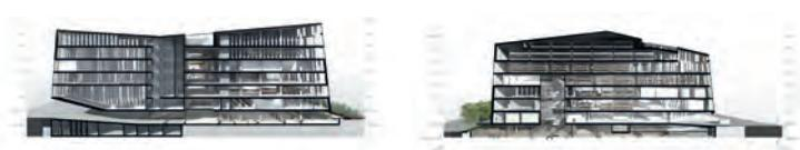
STAVBNI VOLUMEN NATEČAJNE REŠITVE ZAKLJUČUJE OBSTOJEČO OBODNO ZAVIDAVO STAVBNEGA OTOKA, A SE NA OBSTOJEČO STAVBNO STRUKTURU NE NAVEŽE. STAVBA JE KRISTALINSKE OBLINE Z LOMLJENO STREHO IN NAGNjenimi FASADAMI. VHODI V STAVBO SO UREJENI S SEVERA IN VZHODA.
